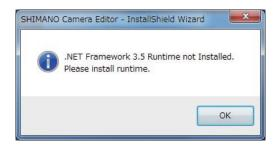
The .NET framework can be configured on the [Turn Windows features on or off] dialog box, accessible as follows: [Control Panel] - [Programs] - [Programs and Features].
